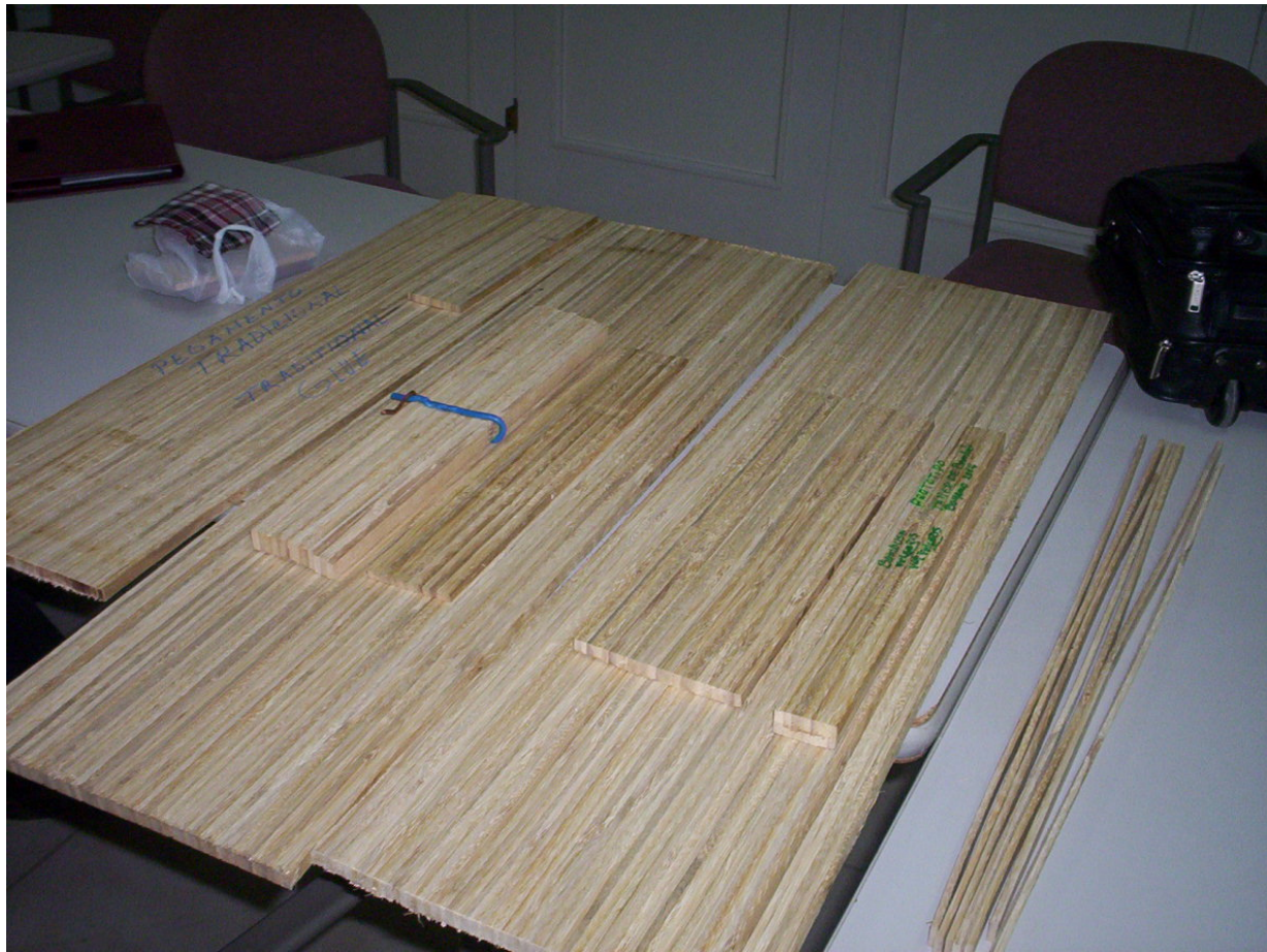
Picture. 3 making of semi manufactured panels with the species Bambusa vulgaris var. vulgaris , in the EFI Bayamo, county Granma.
